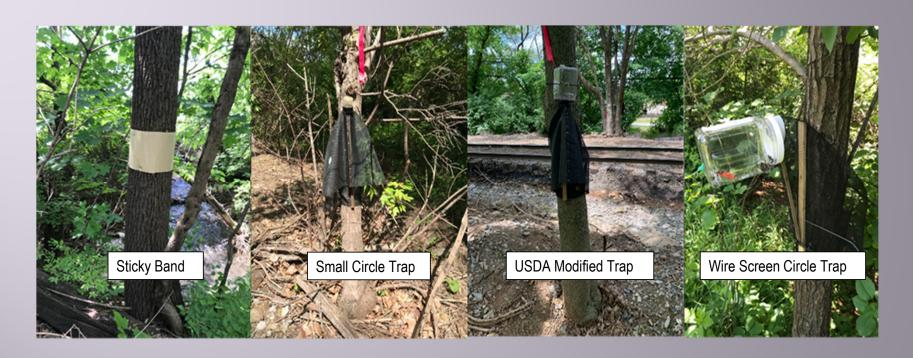
USDA modified traps are the most behaviorally compatible trap design with greatest SLF and fewest non-target captures. No current SLF lures are effective at increasing trap captures. This is an active area of research.
