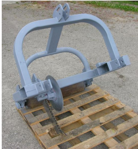
Figure 3 Root pruner designed and constructed by Russell West
