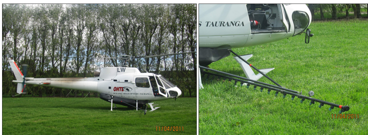
Photo Plate 1: Squirrel Helicopter and nozzle setup on boom
