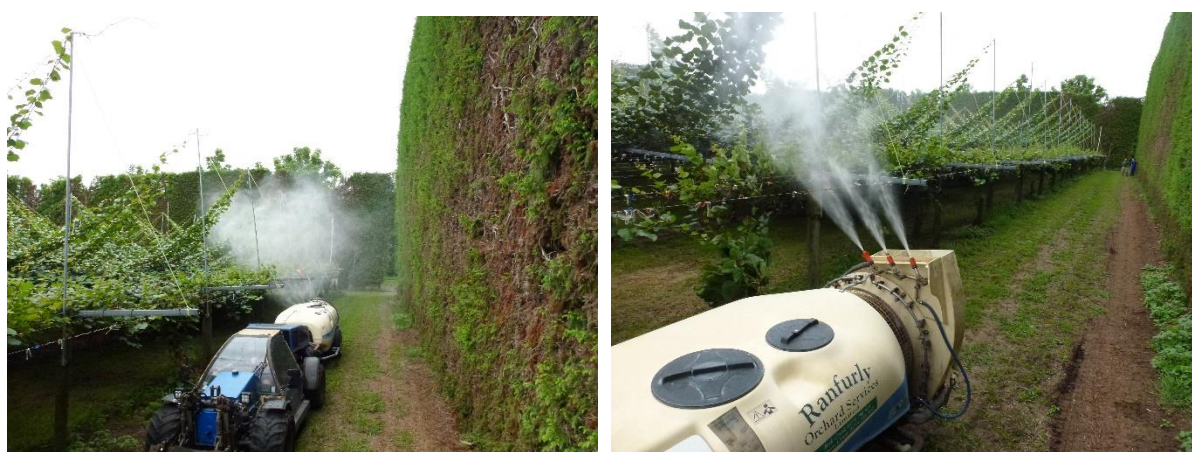
Fig. 3: Standard airblast (LHS) and volute (RHS) spray applications
