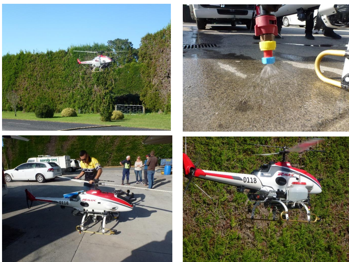
Figure 7: The Yamaha RMax helicopter drone during speed and output swath calibration prior to canopy treatments.
